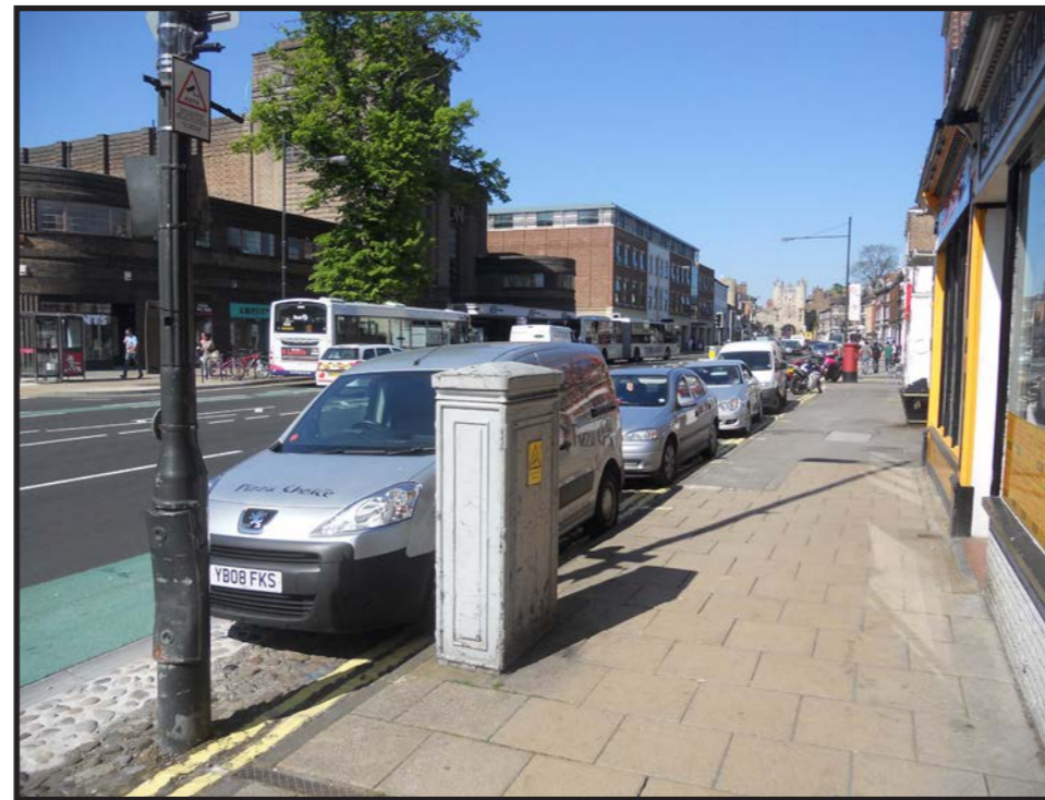
Blossom Street - recently improved through the re-modelling of several pedestrian crossings, improved cycle lanes and the removal of some signage. However, the gateway street contains several types of light column and street furniture is inconsistent. Repair and maintenance of surfaces is also inconsistent and sometimes poor quality.
