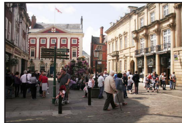
St Helen's Square can be challenging for blind and partially sighted because there is no delineation between footway and carriageway. English Pennine sandstone corduroy edging would significantly damage the square's distinctive character and studs inserted into existing English Pennine sandstone edging may be more appropriate
