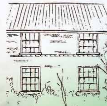
Casement windows & string course at The Limes
