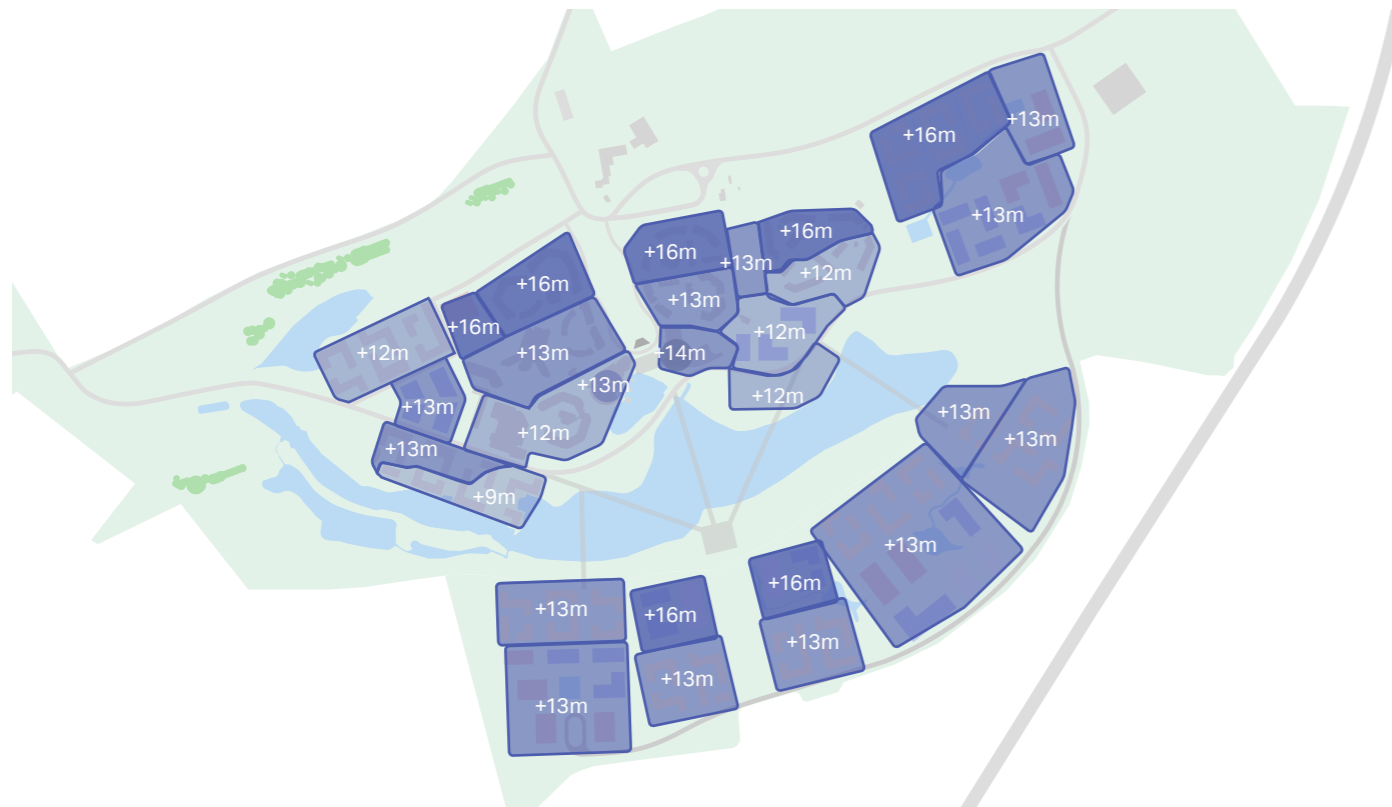
Indicated heights diagram to reflect existing buildings and proposed development relative to grade level. Levels to be read in conjunction with Maximum Building heights diagram within the Master Plan and Strategic Design Brief Document May 2008-2014, which has been reproduced on page 6 of this document
