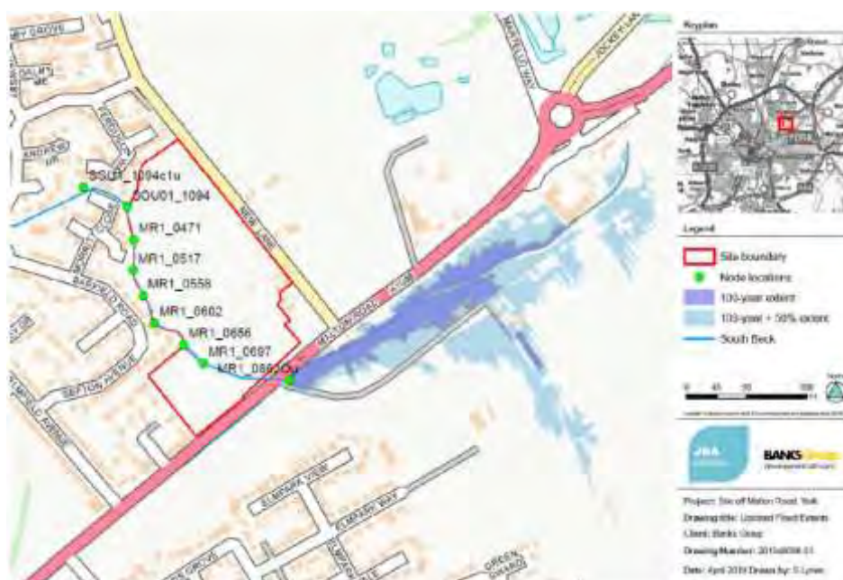
Figure 2: Image from Flood Risk Assessment (2019) highlighting reduced flood risk extent on site.
