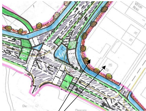
Figure 4.2 Rejected draft design of the Chancery Rise junction improvement on the eastern side of the sub station
